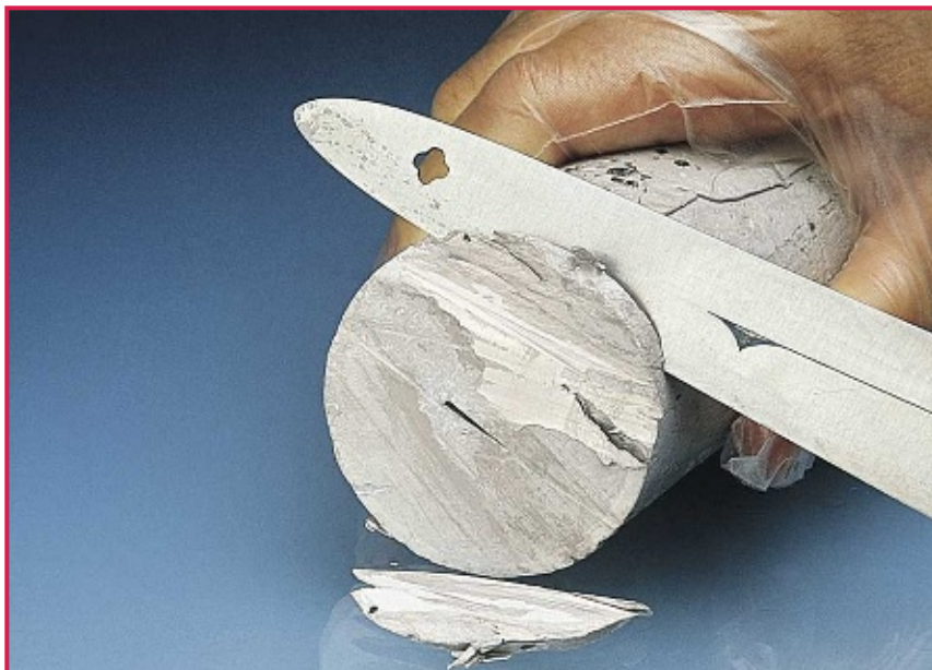
▲ The metal sodium (Na) is soft enough to cut with a knife. It is very reactive, so gloves are used when holding it.
